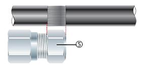
1. Cut back the cable outer sheath to expose the armour to a length not more than the outer nut (5)
